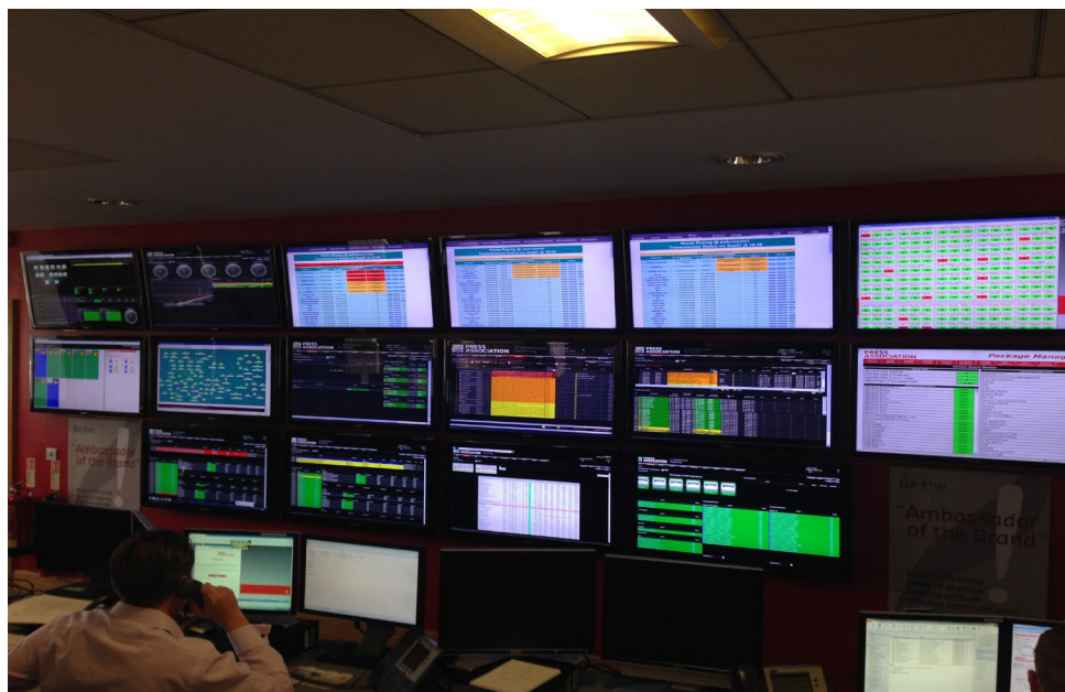
Figure 2. Monitoring Central at Press Association utilizes the customized ScienceLogic dashboards that monitor the entire infrastructure end-to-end as well as all services, feeds, deliverables, and customers.
